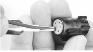
**STEP 1:** Open the CET - SLC extraction tool and place it over the insulation of the wire.
