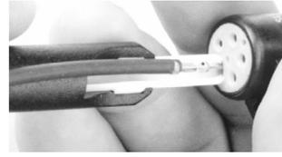
**STEP 3:** While the CET - SLC is bottomed, simply pull the wire/contact assembly out.
