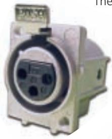
The XLM male and female PCB metal flange mount receptacles offer durability, reliability, space savings, and greatly improved EMI shielding over our plastic XLB-PCB connectors. Ease of installation is enhanced since the grounding terminal can be used to temporarily fasten the connector to the circuit board during assembly. The XLM-PCB connectors are interchangeable and intermateable with our XLR series. RoHS Compliant.
